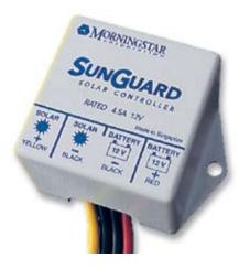
The SunGuard uses the same charging circuit as the SunSaver. It is ideal where a 12-volt low-power controller is needed. It can control up to 75 watts of PV module(s). Since it is epoxy encapsulated, it can be used outdoors in a harsh environment. Dimensions are 2.5" x 2" x 1.6" with wire leads for connecting module and battery. 5-year warranty.
