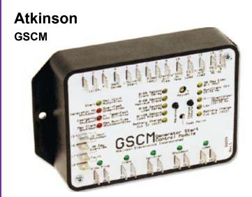
The GSCM (Generator Start Controller Module) is a microprocessor-based generator-starting controller that receives start commands from the 12-volt output from an OutBack FX inverter auxiliary relay, a user-supplied switch, an auxiliary relay in an inverter, a voltage controlled relay, a timer or any user-supplied contact closure. It automatically controls a gas/propane or diesel powered generator or pump, and is totally sealed for harsh environment operation.
