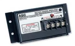
The ASC is a compact, encapsulated, battery charge regulator for use in small photovoltaic systems. It is available in 12-volt and 24-volt units up to 16 amps. The ASC is a switching shunt regulator, housed in an anodized aluminum chassis and encapsulated in a hard epoxy resin. The terminal block accepts up to 12-gauge wire or a spade connector, providing simple installation.
