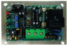
voltage rises to the high setpoint. The relay in the "Active-Low" is powered when voltage drops to the low setpoint. The SPDT relay allows the voltage controlled switch to either connect or disconnect a circuit when it operates or to turn one thing on while turning another thing off.
