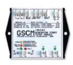
This generator start controller is optimized for use with OutBack inverters. It supports three types of 3-wire gas-generator control: momentary, maintained or ignition. It has a fixed crank time and over and under frequency shutdown.
