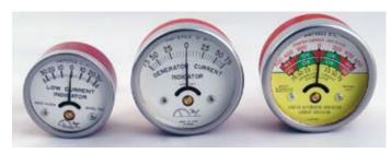
These meters read DC amps from a wire that is placed in the slot frame on the rear of the meter case. No electrical connection is needed. The 30-amp meter will work with wires up to 8 gauge. The dual range meter has a 75-amp scale and a 600-amp scale. This amp meter will work with wire up to 20 gauge.
