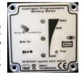
Three LEDs – green, red and yellow – light in various combinations to indicate battery voltage. An audio alarm can be set to sound at high or low voltage levels and all settings are programmable by the user with a push button on the front panel.
