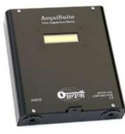
CSV. Data can also be accessed using the modem or LAN connection using any web browser. This enables the user/contractor to push/pull data into energy kiosks, building dashboards, or other custom software applications or web interfaces. The A8812-1 has 8 flex IO inputs; each input can monitor analog, resistance, or pulse data. The AcquiSuite provides a cost-effective solution for monitoring solar system performance down to the string and panel level.
